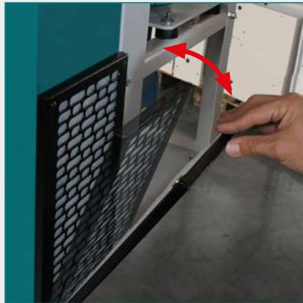
The RS-PRO is optionally available with pre-filter frame to protect against dirt contamination. The frame can be attached very simply by means of magnets.
