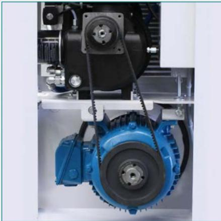
Belt tensioning is effected by means of a motor rocker. The optimum sling arrangement of the belt around the pulley ensures even better power transfer.
