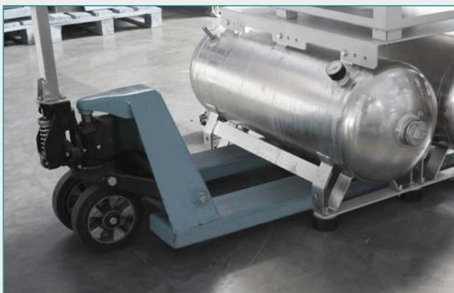
All variants with compressed air tank, manufactured and tested in accordance with AD2000 guidelines, can be moved by a forklift without the need for a pallet.
